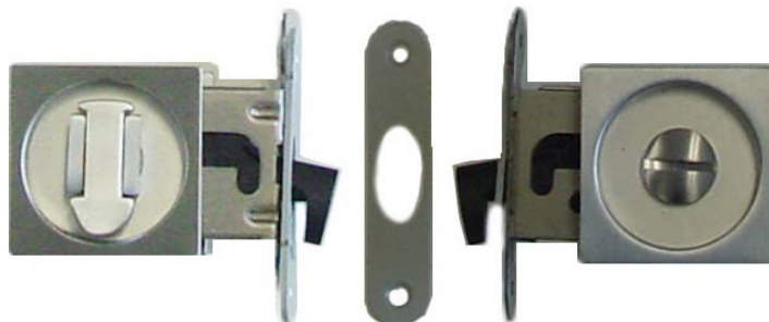
SET: #13.R95; Sliding Lock with Privacy function; Flap lever inside, indicator outside MINIMUM DOOR THICKNESS: 1 1/5" ; size square cups: 2 1/6" x 2 1/16". FOR DETAILS SEE PAGE 1-13-H; 1-13-I and 5-1-C and 5-2-E
