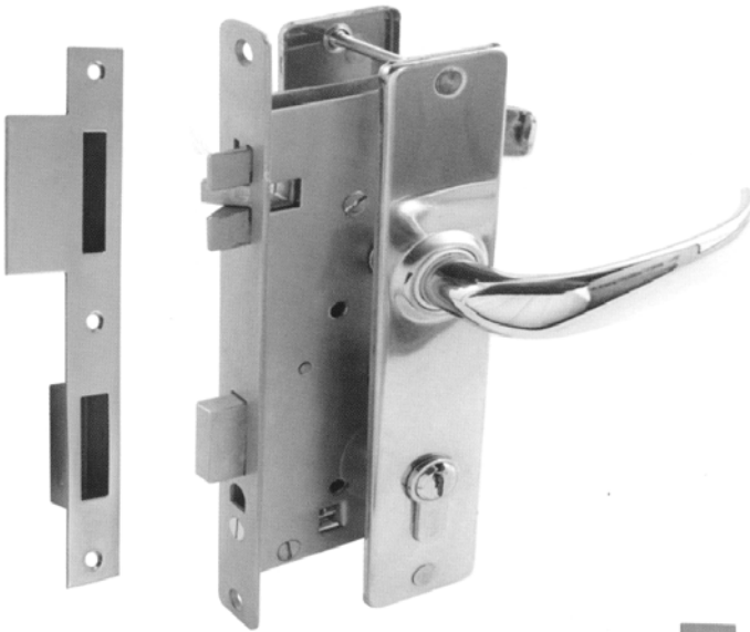
18.2035 SET; Entry Lock; 370 mm backset. Face plate: 212 x 22 x 2 mm; Lock case: 165 high x 75 wide x 13 mm thick. Escutcheon plate: 196 x 38 mm, Lever 110 mm long overall. Marine grade; stainless steel and brass chrome plated parts.
